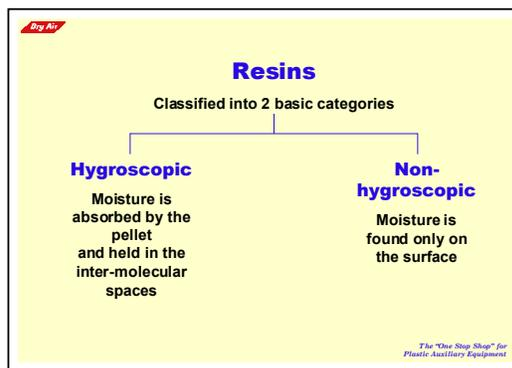
and **absorb moisture** from the **atmosphere** during **storage** or **before being processed**, which **adversely** affects the **final quality** of the moulded part.
