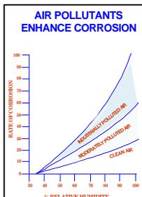
The comparative rates of corrosion in relatively clean and polluted air in shown in the figure. The critical humidity level which is at 45% is approximately same for clear and polluted air, however the rate of corrosion is faster where surfaces are exposed to polluted air in combination with high relative humidity.
